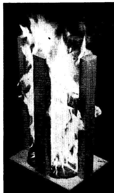
Posts B, B', C, C', 1 1/2 x 2 1/2 x 24 inches; bar D, 1 1/2 x 2 1/2 x 12 inches; bar E, 1 1/2 x 2 1/2 x 7 inches
